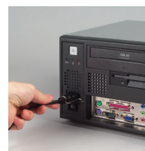
Plug ring-lock securely fastens the power cord
